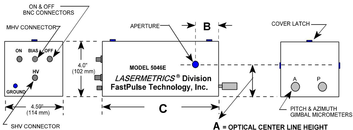
**Figure 3: OPTICAL HEAD ASSEMBLY
