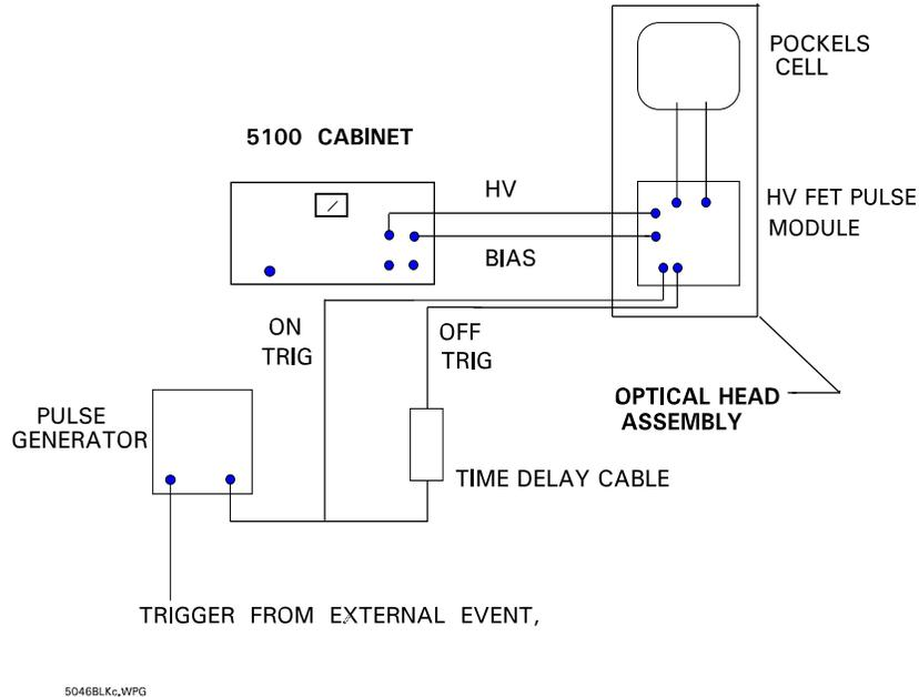
**Figure 8 DIRECT TRIGGERING OF HV MODULES (In the 5100EMW Optical Head Assembly)**
