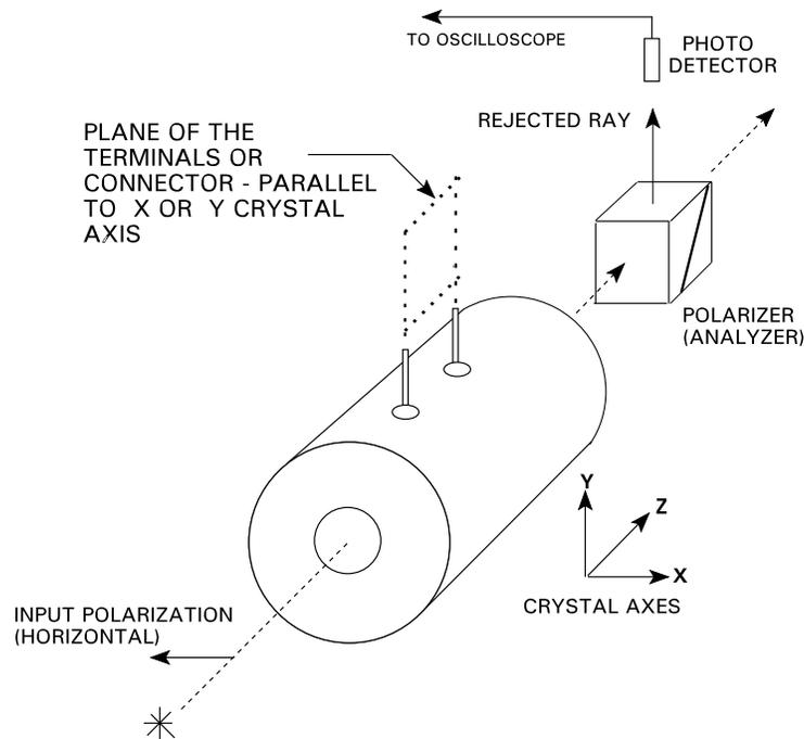
Figure 9. Arrangement of elements for detecting laser pulses with no voltages applied. Shows orientation of Pockels cell terminals with incoming plane of polarization. If the input plane of polarization is vertical and the cell is not rotated, the output polarizer (analyzer) can be rotated  $90^\circ$  around the propagation axis and operation will be identical. Typically, the X and Y crystallographic axes are optically equal and interchangeable.
