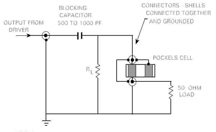
Figure 9: Circuit for blocking DC voltage from being applied to the crystal and approximating a 50 Ohm load
