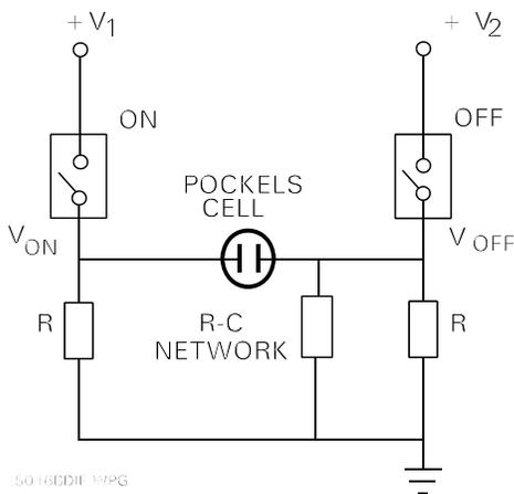
Figure 13: Differential Pulse Driver
