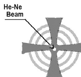
Figure 2: Isogyre pattern with beam centered
