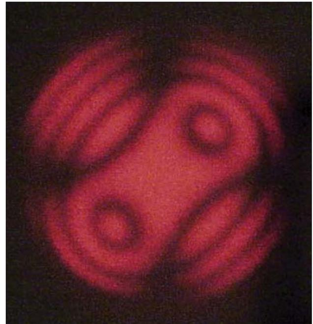
Half Wave Voltage,  $\sim 3.8$  kVDC Applied
