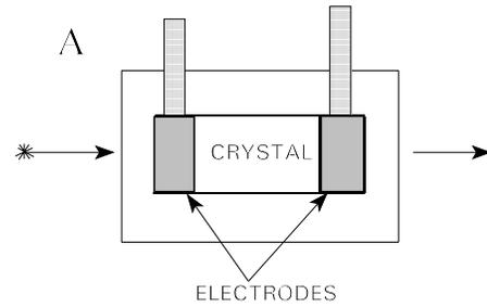
Configuration B: Suitable for transmission line applications. The "straight through" arrangement allows attachment of the driving cable to one side of the Pockels cell and an output cable to the opposite side. The output cable is usually terminated with a resistor which matches the cable characteristic impedance, thus preventing electrical reflections.
