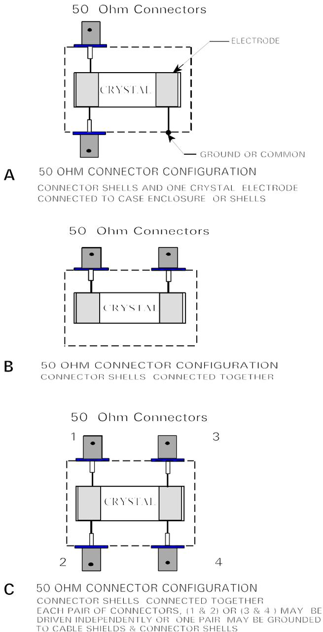
Figure 8: Pockels Cells with 50 Ω Connectors
