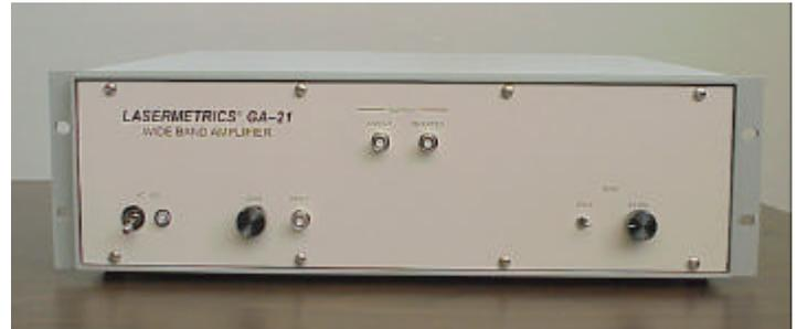
High frequency response of the GA-21R is a function of the load capacitance which includes the modulator and interconnecting coaxial cables.
